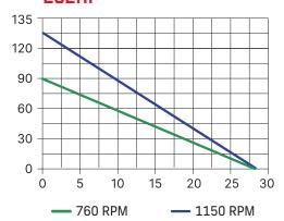
DRIVER RPM: 1800 DRIVEN RPM: 760 HORSEPOWER: 5 TYPE: Rotary vane
