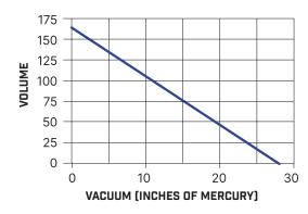
DRIVER RPM: 1800 DRIVEN RPM: 850 HORSEPOWER: 10 TYPE: Rotary vane
