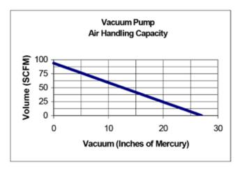
Driver RPM: 1800 Driven RPM: 850 Horsepower: 5 Type: Rotary Vane
